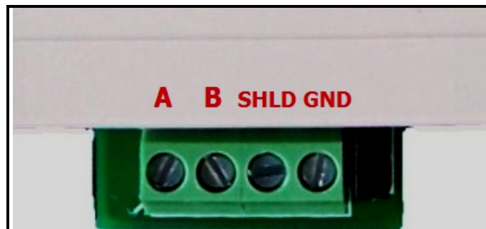
Figure 9: RS-485 Connection Terminals
